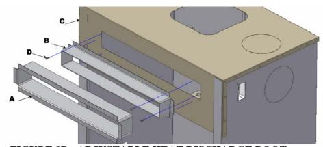
FIGURE 9B: ADJUSTABLE HEAT DISCHARGE BOOT (OPTIONAL)
